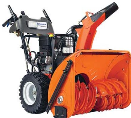
**ДВИГАТЕЛЬ:** Briggs&Stratton 1650 Snow Max Series; OHV; 342 см<sup>3</sup>
